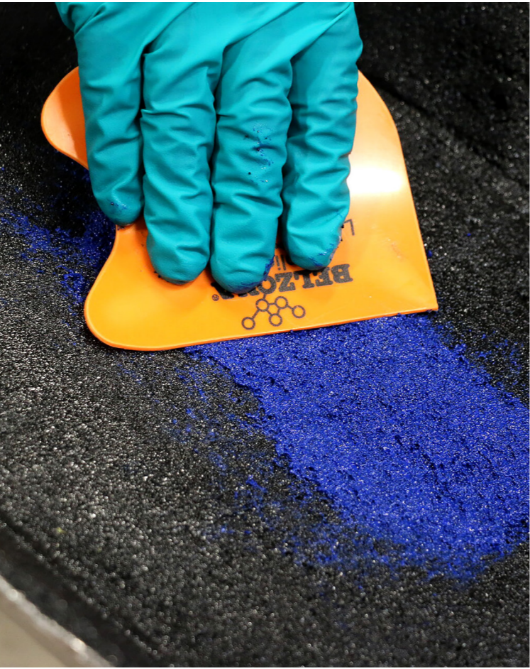
Belzona 1818 Fast-curing, surface-tolerant abrasion and wear-resistant epoxy repair composite, suitable for emergency repairs.
