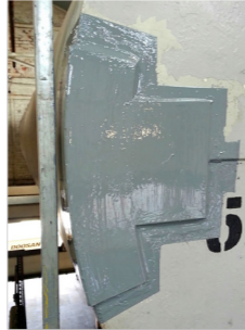
Belzona 1212 High-performance, rapid-curing, surface-tolerant epoxy repair composite suitable for wet and oily surfaces. Approved for contact with drinking water (e.g. WRAS).
