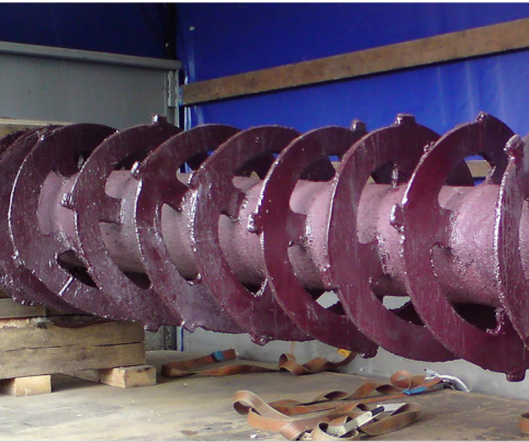
Belzona 1811 (Ceramic Carbide) Ceramic-filled high abrasion and wear-resistant epoxy repair composite, particularly suitable for large particle abrasion.
