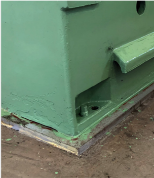
Belzona 7111 Pourable chocking/grouting material designed to spread evenly across uneven surfaces to endure physical and thermal shock.
