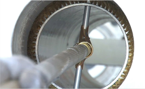
Belzona 1331 Sprayable, erosion-corrosion-resistant epoxy coating with ultra-high molecular weight polymer fillers. Approved for contact with drinking water (e.g. WRAS).
