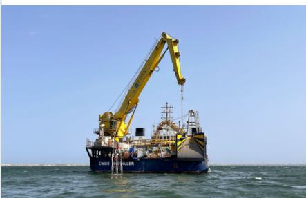
Cable layer CMOS-INSTALLER for the installation of two submarine power cables in Dakar, Senegal.
